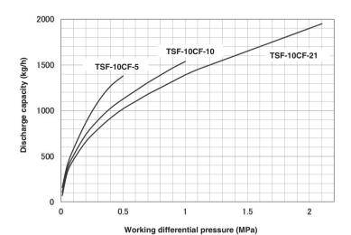
The discharge capacity shown in the charts on the above is the maximum value. In designing a system, select a steam trap with a sufficient safety factor (more than two times the regular level).
